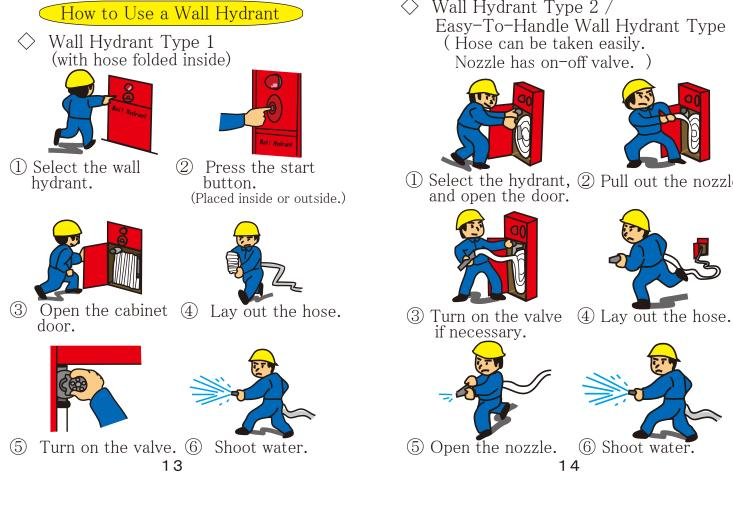
◇ Wall Hydrant Type 2 / Easy-To-Handle Wall Hydrant Type 1 (Hose can be taken easily. Nozzle has on-off valve. )
